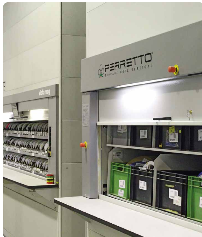
Rotating storage systems for integrated circuit components
