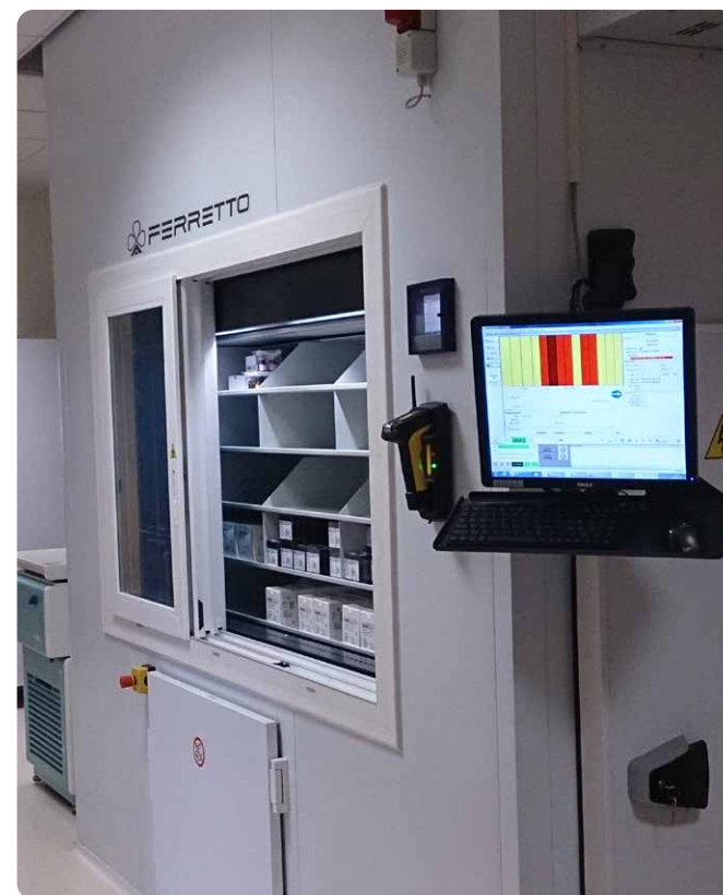
Temperature-controlled rotating storage systems (Hospital Sector)
